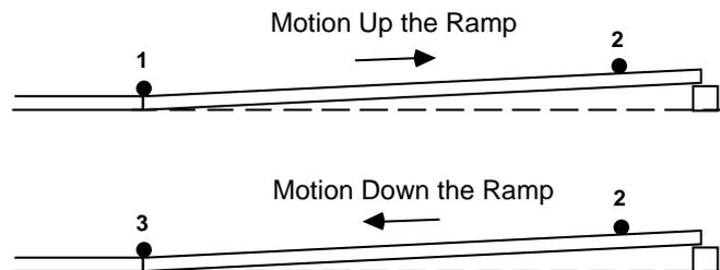
A steel ball is launched with some initial velocity, slows down as it travels up a gentle incline, reverses direction, and then speeds up as it returns to its starting point. Assume friction is negligible.
